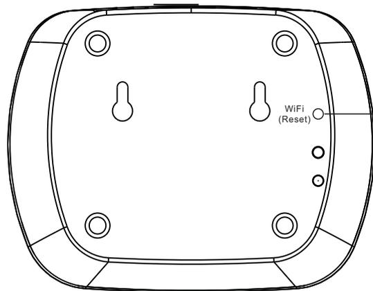
WiFi Reset switch: press and hold down for 10S then release, the blue WiFi indicator will go off and go on again, WiFi setting will be factory reset.
